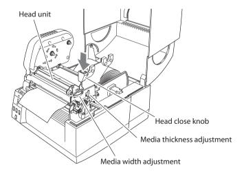
9. With the power switched on, push the FEED key to feed the media.
