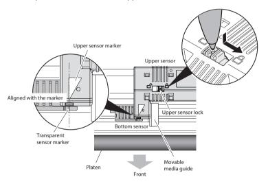
When using media that is 4 inches wide, position the upper sensor and the bottom sensor all the way to the right (large blue-head open lever side).
