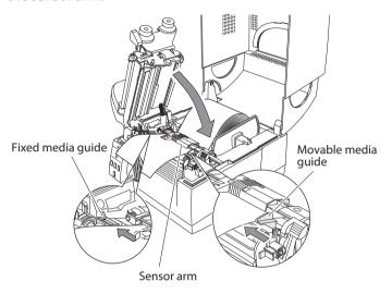
Media Thickness Adjustment(P.48) Media Width Adjustment(P.49) 8. Push the head close knob to lower and lock the head unit. Be sure to always push the head close knob to lock the head unit. Align it with the width of the media that has been set, then set the media width and media thickness adjustment dials. See "Chapter 3 Printer Adjustments".
