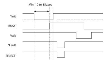
**Note:** If the \*Init signal does not have width of 10 to 15µsec or more, it cannot act as an Init signal. If it is lower, the \*Init signal is ignored. BUSY starts up when the \*Init signal is perceived.
