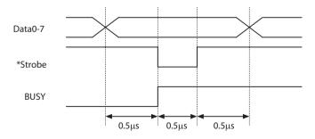
**Note:** Busy rises when \*Strobe signal starts, and data is latched with \*Strobe signal starts.
